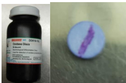
Figure 8: Purple Colour Observed 5 Minutes after Culture was Streaked on Oxidase Disc
